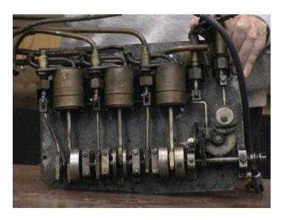
single acting piston valve engine. A wall mountable unit originally from a boat of about eight feet in length. The unit has no castings, six main bearings and a built up crankshaft. ran sweetly on the air supply, drawing gasps admiration of from the quiet attentive and audience.
